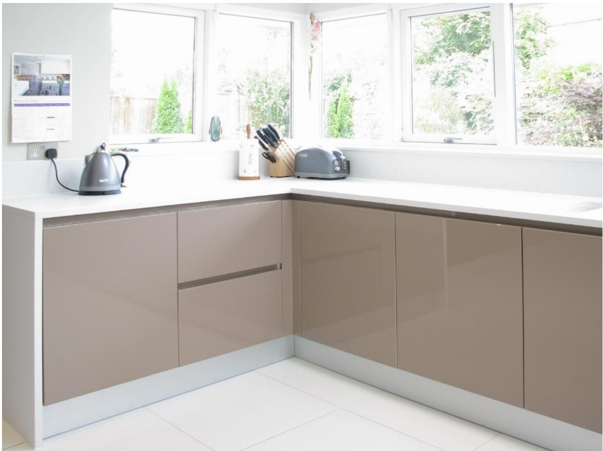
The Oaks, Foxrock, Kitchen design coffee coloured, 7 layer high gloss lacquer polyester finish, handle less, in combination with leather finish Silestone worktop
